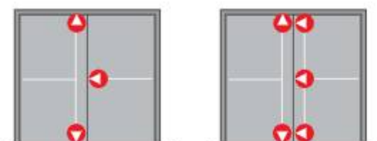
Three point locking over rebated door
